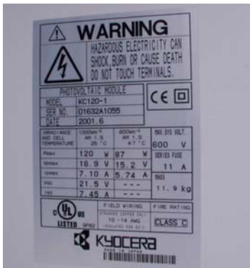
Figure 1 PV Module Listing Label
