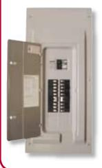
Just like the electrical circuits in your home or office, an inverter's electrical output needs to be routed through an AC circuit breaker. This breaker is usually mounted inside the building's mains panel, which enables the inverter to be disconnected from either the grid or from electrical loads if servicing is necessary, and also safeguards the circuit's electrical wiring.
