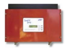
Most grid-intertie inverters can be installed outdoors (ideally, in the shade). Most off-grid inverters are not weatherproof and should be mounted indoors, close to the battery bank.
